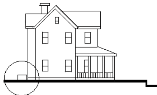
Inappropriate Avoid the installation of mechanical equipment on the street facade.
