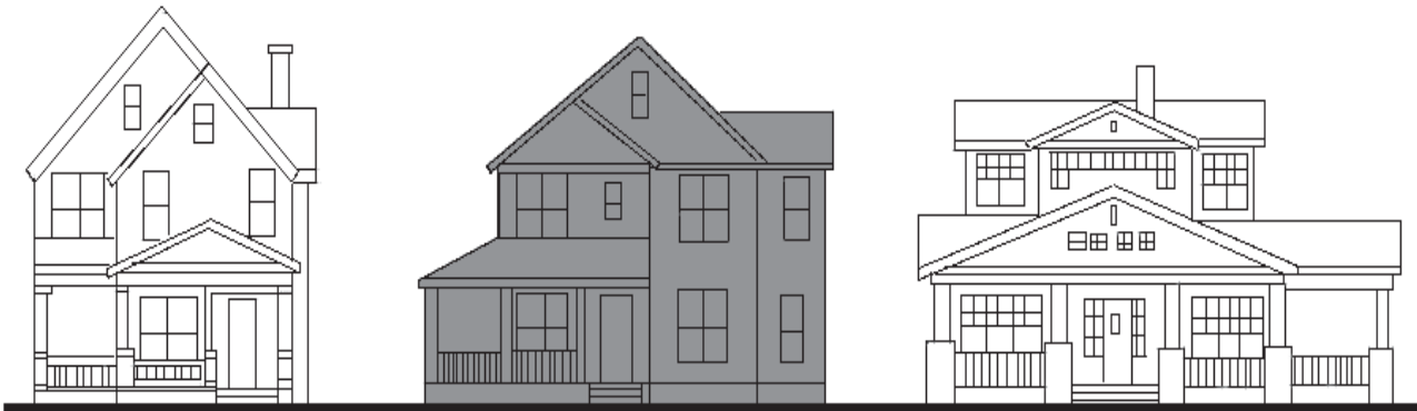
Appropriate Spacing, placement, scale, orientation and scale of windows in the new construction are compatible with the surrounding buildings.
