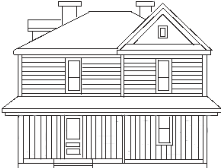
Inappropriate Siding should be applied horizontally.
